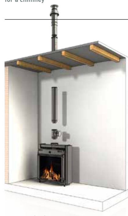
Via the roof (flat) • direct or with the pipe bends
