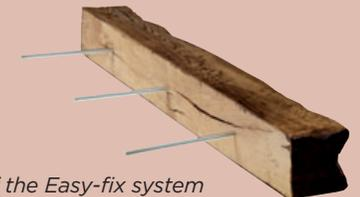
If the Easy-fix system is not specified: we supply three M10 x 300mm threaded metal bars that screw into pre-drilled holes in the back of the beam. The wall should then be drilled with 12mm holes to accept these bars. You will need to provide your own additional adhesives.
